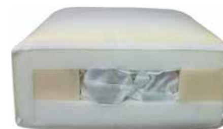
Luxury Spring Seat (LSS) - A cushion that features a Marshall spring unit which is encased in a high resiliency urethane core. Then a soft-cell foam layer is applied to the top and bottom and is sewn into a ticking.
